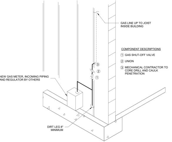
5 PIPING - GAS METER CONNECTION, ISO NTS
