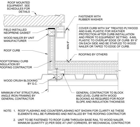
1 HVAC - EQUIPMENT - RTU / MAU CURB DETAIL NTS
