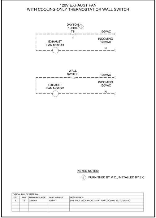
7 WIRING - 120V EF WITH THERMOSTAT NTS
