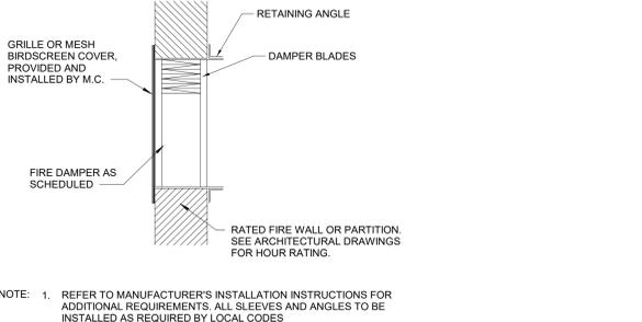
9 HVAC - LIFE SAFETY, FIRE DAMPER, W/O DUCT CONNECTION NTS
