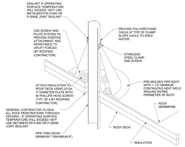
6 PIPING - PIPE THRU ROOF NTS
